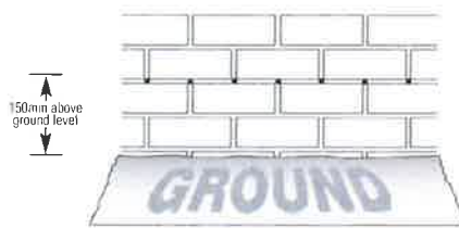
Figure 9: Drilling pattern for Stretching Bond
